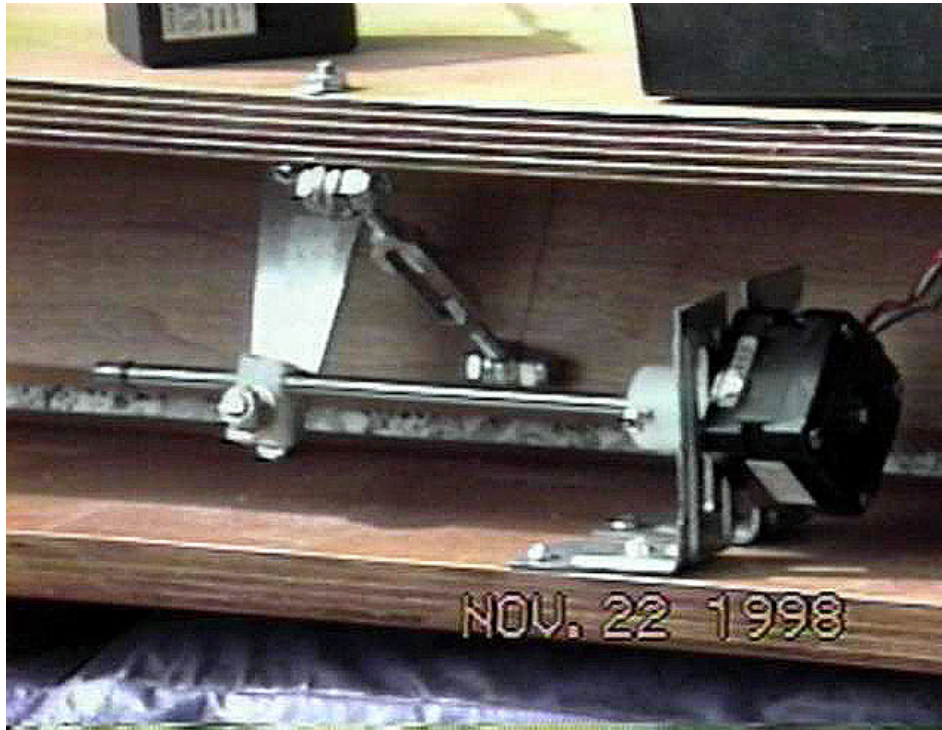
Closeup of the original motor, bracket and T hinge...
