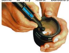
eyepieces definitely looked scratch free and very squeaky clean. The only drawback I could see to this device was the fact that it left a small amount of dry residue on the surface of the lens after cleaning was complete. This residue was in the form of small particles of carbon, the LensPen's cleaning compound, and was easily brushed away.
